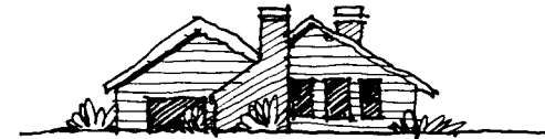
Break roof lines and forms to reflect the irregular forms of the surroundings.
