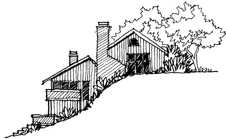
Step building to conform to site topography
